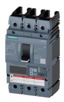
circuit breaker 3VA6 UL frame 150 breaking capacity class M 35kA @ 480V 3-pole, line protection ETU830, LIG, In=150A overload protection Ir=60A...150A short-circuit protection Ii=1.5...10 x In ground-fault protection Ig=0.2...1 x In, tg=0.05-0.8s without connection
