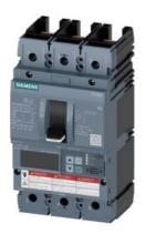
Circuit breaker 3VA6 UL Frame 150 breaking capacity class M 35kA @ 480V 3-pole, Line protection ETU560, LSIG, In=150A overload protection, 100% rated Ir=60A...150A Short-circuit protection Isd=0.6..10x In, Ii=1.5..10x In N conductor protection optionally with external CT, up to 160% Ground-fault protection Ig=0.2...1 x In, tg=0.05-0.8s without connection
