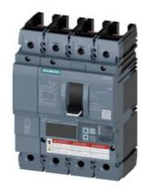
Circuit breaker 3VA6 UL Frame 150 breaking capacity class C 100kA @ 480V 4-pole, Line protection ETU856, LSI, In=100A overload protection, 100% rated Ir=40A...100A Short-circuit protection Isd=0.6..10x In, Ii=1.5..12x In N conductor protection adjustable (OFF, up to 150%) Ground-fault alarm message via EFB300 or COM without connection
