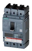
Circuit breaker 3VA6 UL Frame 150 breaking capacity class C 100kA @ 480 V 3-pole, Line protection ETU856, LSI, In=100A overload protection, 100% rated Ir=40A ...100A Short-circuit protection Isd=0.6..10x In, Ii=1.5..12x In N conductor protection optionally with external CT; up to 160% Ground-fault alarm message via EFB300 or COM nut keeper kit on both sides
