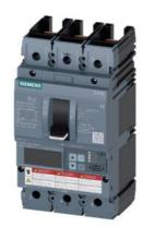
Circuit breaker 3VA6 UL Frame 150 breaking capacity class C 100kA @ 480V 3pole, Line protection ETU856, LSI, In=100A overload protection, 100% rated Ir=40A...100A Short-circuit protection Isd=0.6..10x In, Ii=1.5..12x In N conductor protection optionally with external CT, up to 160% Ground-fault alarm message via EFB300 or COM without connection
