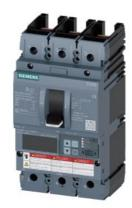
circuit breaker 3VA6 UL frame 150 breaking capacity class C 100kA @ 480V 3pole, line protection ETU856, LSI, In=100A overload protection Ir=40A...100A short-circuit protection Isd=0.6..10x In, Ii=1.5..12x In N conductor protection optionally with external current transformer, up to 160% ground-fault alarm message via EFB300 or COM without connection
