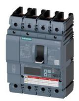
Circuit breaker 3VA6 UL Frame 150 breaking capacity class C 100kA @ 480V 4-pole, Line protection ETU860, LSIG, In=100A overload protection, 100% rated Ir=40A...100A Short-circuit protection Isd=0.6..10x In, Ii=1.5..12x In N conductor protection adjustable (OFF, up to 150%) Ground-fault protection Ig=0.2...1 x In= tg=0.05-0.8s without connection
