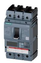
Circuit breaker 3VA6 UL Frame 150 breaking capacity class C 100kA @ 480 V 3-pole, Line protection ETU860, LSIG, In=100A overload protection, 100% rated Ir=40A ...100A Short-circuit protection Isd=0.6..10x In, Ii=1.5..12x In N conductor protection optionally with external CT; up to 160% Ground-fault protection Ig=0.2... 1 x In, tg=0.05-0.8s nut keeper kit on both sides
