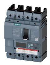
Circuit breaker 3VA6 UL Frame 150 breaking capacity class C 100kA @ 480V 4-pole, Line protection ETU850, LSI, ln=100A overload protection, 100% rated lr=40A...100A Short-circuit protection lsd=0.6..10x ln, li=1.5..12x ln N conductor protection adjustable (OFF, up to 150%) without connection
