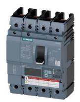
Circuit breaker 3VA6 UL Frame 150 breaking capacity class C 100kA @ 480V 4-pole, Line protection ETU830, LIG, In=100A overload protection, 100% rated Ir=40A...100A Short-circuit protection Ii=1.5...12 x In Ground-fault protection Ig=0.2...1 x In, tg=0.05-0.8s without connection
