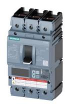
Circuit breaker 3VA6 UL Frame 150 breaking capacity class C 100kA @ 480 V 3pole, Line protection ETU830, LIG, In=100A overload protection, 100% rated Ir=40A ...100A Short-circuit protection Ii=1.5...12 x In Ground-fault protection Ig=0.2... 1 x In, tg=0.05-0.8s cable connection on both sides
