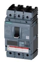
Circuit breaker 3VA6 UL Frame 150 breaking capacity class C 100kA @ 480 V 3pole, Line protection ETU830, LIG, In=100A overload protection, 100% rated Ir=40A ...100A Short-circuit protection Ii=1.5...12 x In Ground-fault protection Ig=0.2... 1 x In, tg=0.05-0.8s nut keeper kit on both sides
