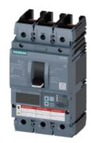
circuit breaker 3VA6 UL frame 150 breaking capacity class C 100kA @ 480V 3-pole, line protection ETU830, LIG, In=100A overload protection Ir=40A...100A short-circuit protection Ii=1.5...12 x In ground-fault protection Ig=0.2...1 x In, tg=0.05-0.8s without connection
