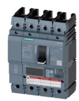
Circuit breaker 3VA6 UL Frame 150 breaking capacity class C 100kA @ 480V 4-pole, Line protection ETU820, LI, In=100A overload protection, 100% rated Ir=40A...100A Short-circuit protection Ii=1.5...12 x In without connection
