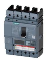
Circuit breaker 3VA6 UL Frame 150 breaking capacity class C 100kA @ 480V 4-pole, Line protection ETU556, LSI, In=100A overload protection, 100% rated Ir=40A...100A Short-circuit protection Isd=0.6..10x In, Ii=1.5..12x In N conductor protection adjustable (OFF, up to 150%) Ground-fault alarm message via EFB300 or COM without connection
