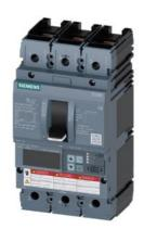
Circuit breaker 3VA6 UL Frame 150 breaking capacity class C 100kA @ 480 V 3-pole, Line protection ETU556, LSI, In=100A overload protection, 100% rated Ir=40A ...100A Short-circuit protection Isd=0.6..10x In, Ii=1.5..12x In N conductor protection optionally with external CT; up to 160% Ground-fault alarm message via EFB300 or COM nut keeper kit on both sides
