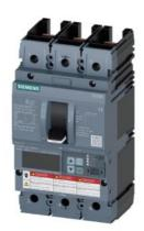
Circuit breaker 3VA6 UL Frame 150 breaking capacity class C 100kA @ 480V 3-pole, Line protection ETU556, LSI, In=100A overload protection, 100% rated Ir=40A...100A Short-circuit protection Isd=0.6..10x In, Ii=1.5..12x In N conductor protection optionally with external CT, up to 160% Ground-fault alarm message via EFB300 or COM without connection
