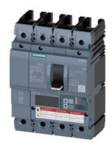
Circuit breaker 3VA6 UL Frame 150 breaking capacity class C 100kA @ 480V 4-pole, Line protection ETU560, LSIG, In=100A overload protection, 100% rated Ir=40A...100A Short-circuit protection Isd=0.6..10x In, Ii=1.5..12x In N conductor protection adjustable (OFF, up to 150%) Ground-fault protection Ig=0.2...1 x In= tg=0.05-0.8s without connection
