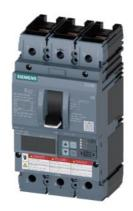
Circuit breaker 3VA6 UL Frame 150 breaking capacity class C 100kA @ 480 V 3-pole, Line protection ETU560, LSIG, In=100A overload protection, 100% rated Ir=40A ...100A Short-circuit protection Isd=0.6..10x In, Ii=1.5..12x In N conductor protection optionally with external CT; up to 160% Ground-fault protection Ig=0.2... 1 x In, tg=0.05-0.8s nut keeper kit on both sides
