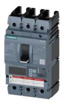
circuit breaker 3VA6 UL frame 150 breaking capacity class C 100kA @ 480V 3-pole, line protection ETU550, LSI, In=100A overload protection Ir=40A...100A short-circuit protection Isd=0.6..10x In, Ii=1.5..12x In N conductor protection optionally with external current transformer, up to 160% without connection
