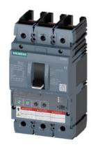
Circuit breaker 3VA6 UL Frame 150 breaking capacity class C 100kA @ 480V 3-pole, Line protection ETU350, LSI, In=100A overload protection, 100% rated Ir=40A...100A Short-circuit protection Isd=1.5...10 x Ir, Ii=12 x In without connection
