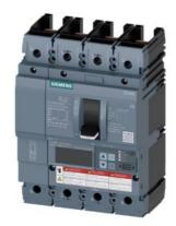
Circuit breaker 3VA6 UL Frame 150 breaking capacity class H 65kA @ 480V 4-pole, Line protection ETU856, LSI, In=100A overload protection, 100% rated Ir=40A...100A Short-circuit protection Isd=0.6..10x In, Ii=1.5..12x In N conductor protection adjustable (OFF, up to 150%) Ground-fault alarm message via EFB300 or COM without connection
