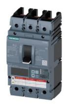
circuit breaker 3VA6 UL frame 150 breaking capacity class H 65kA @ 480V 3-pole, line protection ETU856, LSI, In=100A overload protection Ir=40A...100A shortcircuit protection Isd=0.6..10x In, Ii=1.5..12x In N conductor protection optionally with external current transformer, up to 160% ground-fault alarm message via EFB300 or COM without connection
