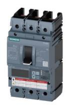
Circuit breaker 3VA6 UL Frame 150 breaking capacity class H 65kA @ 480V 3-pole, Line protection ETU850, LSI, In=100A overload protection, 100% rated Ir=40A...100A Short-circuit protection Isd=0.6..10x In, Ii=1.5..12x In N conductor protection optionally with external CT, up to 160% without connection
