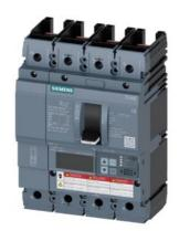
Circuit breaker 3VA6 UL Frame 150 breaking capacity class H 65kA @ 480V 4-pole, Line protection ETU830, LIG, In=100A overload protection, 100% rated Ir=40A...100A Short-circuit protection Ii=1.5...12 x In Ground-fault protection Ig=0.2...1 x In, tg=0.05-0.8s without connection
