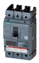
Circuit breaker 3VA6 UL Frame 150 breaking capacity class H 65kA @ 480V 3-pole, Line protection ETU830, LIG, In=100A overload protection, 100% rated Ir=40A...100A Short-circuit protection Ii=1.5...12 x In Ground-fault protection Ig=0.2...1 x In, tg=0.05-0.8s without connection
