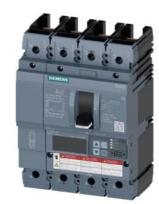
Circuit breaker 3VA6 UL Frame 150 breaking capacity class H 65kA @ 480V 4pole, Line protection ETU550, LSI, In=100A overload protection, 100% rated Ir=40A...100A Short-circuit protection Isd=0.6..10x In, Ii=1.5..12x In N conductor protection adjustable (OFF, up to 150%) without connection
