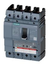
Circuit breaker 3VA6 UL Frame 150 breaking capacity class H 65kA @ 480V 4-pole, Line protection ETU350, LSI, In=100A overload protection, 100% rated Ir=40A...100A Short-circuit protection Isd=1.5...10 x Ir, Ii=12 x In N conductor protection adjustable (OFF, 50%, 100%) without connection
