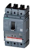
Circuit breaker 3VA6 UL Frame 150 breaking capacity class H 65kA @ 480V 3-pole, Line protection ETU330, LIG, In=100A overload protection, 100% rated Ir=40A...100A Short-circuit protection Ii=1.5...12 x In Ground-fault protection Ig=0.2...1 x In, tg=0.1/0.3s without connection
