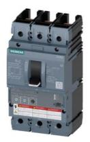
Circuit breaker 3VA6 UL Frame 150 breaking capacity class H 65kA @ 480V 3-pole, Line protection ETU320, LI, In=100A overload protection, 100% rated Ir=40A...100A Short-circuit protection Ii=1.5...12 x In without connection
