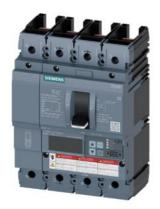
Circuit breaker 3VA6 UL Frame 150 breaking capacity class M 35kA @ 480V 4-pole, Line protection ETU856, LSI, In=100A overload protection, 100% rated Ir=40A...100A Short-circuit protection Isd=0.6..10x In, Ii=1.5..12x In N conductor protection adjustable (OFF, up to 150%) Ground-fault alarm message via EFB300 or COM without connection
