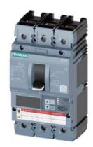
circuit breaker 3VA6 UL frame 150 breaking capacity class M 35kA @ 480 V 3pole, line protection ETU856, LSI, In=100A overload protection Ir=40A ...100A short-circuit protection Isd=0.6..10x In, Ii=1.5..12x In N conductor protection opt. w. ext. CT; up to 160% ground-fault alarm message via EFB300 or COM cable connection on both sides
