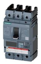
Circuit breaker 3VA6 UL Frame 150 breaking capacity class M 35kA @ 480V 3-pole, Line protection ETU856, LSI, In=100A overload protection, 100% rated Ir=40A...100A Short-circuit protection Isd=0.6..10x In, Ii=1.5..12x In N conductor protection optionally with external CT, up to 160% Ground-fault alarm message via EFB300 or COM without connection
