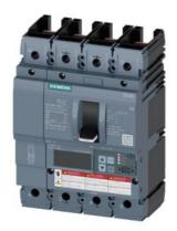
Circuit breaker 3VA6 UL Frame 150 breaking capacity class M 35kA @ 480V 4-pole, Line protection ETU850, LSI, In=100A overload protection, 100% rated Ir=40A...100A Short-circuit protection Isd=0.6..10x In, Ii=1.5..12x In N conductor protection adjustable (OFF, up to 150%) without connection
