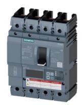
circuit breaker 3VA6 UL frame 150 breaking capacity class M 35kA @ 480V 4-pole, line protection ETU830, LIG, In=100A overload protection Ir=40A...100A short-circuit protection Ii=1.5...12 x In ground-fault protection Ig=0.2...1 x In, tg=0.05-0.8s without connection
