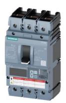
Circuit breaker 3VA6 UL Frame 150 breaking capacity class M 35kA @ 480 V 3-pole, Line protection ETU830, LIG, In=100A overload protection, 100% rated Ir=40A ...100A Short-circuit protection Ii=1.5...12 x In Ground-fault protection Ig=0.2... 1 x In, tg=0.05-0.8s cable connection on both sides
