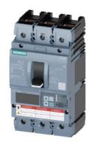
circuit breaker 3VA6 UL frame 150 breaking capacity class M 35kA @ 480 V 3-pole, line protection ETU830, LIG, In=100A overload protection Ir=40A ...100A short-circuit protection Ii=1.5...12 x In ground-fault protection Ig=0.2... 1 x In, tg=0.05-0.8s cable connection on both sides
