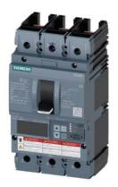
Circuit breaker 3VA6 UL Frame 150 breaking capacity class M 35kA @ 480V 3-pole, Line protection ETU830, LIG, In=100A overload protection, 100% rated Ir=40A...100A Short-circuit protection Ii=1.5...12 x In Ground-fault protection Ig=0.2...1 x In, tg=0.05-0.8s without connection
