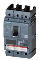
circuit breaker 3VA6 UL frame 150 breaking capacity class M 35kA @ 480V 3-pole, line protection ETU830, LIG, In=100A overload protection Ir=40A...100A short-circuit protection Ii=1.5...12 x In ground-fault protection Ig=0.2...1 x In, tg=0.05-0.8s without connection
