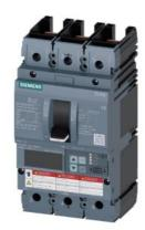
Circuit breaker 3VA6 UL Frame 150 breaking capacity class M 35kA @ 480V 3pole, Line protection ETU556, LSI, In=100A overload protection, 100% rated Ir=40A...100A Short-circuit protection Isd=0.6..10x In, Ii=1.5..12x In N conductor protection optionally with external CT, up to 160% Ground-fault alarm message via EFB300 or COM without connection
