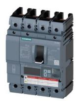
Circuit breaker 3VA6 UL Frame 150 breaking capacity class M 35kA @ 480V 4-pole, Line protection ETU560, LSIG, In=100A overload protection, 100% rated Ir=40A...100A Short-circuit protection Isd=0.6..10x In, Ii=1.5..12x In N conductor protection adjustable (OFF, up to 150%) Ground-fault protection Ig=0.2...1 x In=tg=0.05-0.8s without connection
