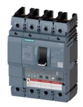
Circuit breaker 3VA6 UL Frame 150 breaking capacity class M 35kA @ 480V 4-pole, Line protection ETU330, LIG, In=100A overload protection, 100% rated Ir=40A...100A Short-circuit protection Ii=1.5...12 x In N conductor protection adjustable (OFF, 50%, 100%) Ground-fault protection Ig=0.2...1 x In= tg=0.1/0.3s without connection
