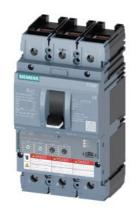
Circuit breaker 3VA6 UL Frame 150 breaking capacity class M 35kA @ 480 V 3pole, Line protection ETU330, LIG, In=100A overload protection, 100% rated Ir=40A ...100A Short-circuit protection li=1.5...12 x In Ground-fault protection Ig=0.2... 1 x In, tg=0.1/0.3s cable connection on both sides
