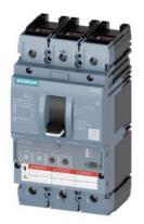
circuit breaker 3VA6 UL frame 150 breaking capacity class M 35kA @ 480 V 3-pole, line protection ETU330, LIG, ln=100A overload protection lr=40A ...100A short-circuit protection li=1.5...12 x ln ground-fault protection lg=0.2... 1 x ln, tg=0.1/0.3s cable connection on both sides
