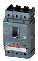
Circuit breaker 3VA6 UL Frame 150 breaking capacity class M 35kA @ 480 V 3-pole, Line protection ETU330, LIG, In=100A overload protection, 100% rated Ir=40A ...100A Short-circuit protection Ii=1.5...12 x In Ground-fault protection Ig=0.2... 1 x In, tg=0.1/0.3s nut keeper kit on both sides
