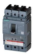
circuit breaker 3VA6 UL frame 150 breaking capacity class M 35kA @ 480 V 3-pole, line protection ETU330, LIG, ln=100A overload protection lr=40A ...100A short-circuit protection li=1.5...12 x ln ground-fault protection lg=0.2... 1 x ln, tg=0.1/0.3s nut keeper kit on both sides
