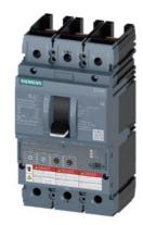
Circuit breaker 3VA6 UL Frame 150 breaking capacity class M 35kA @ 480V 3-pole, Line protection ETU330, LIG, In=100A overload protection, 100% rated Ir=40A...100A Short-circuit protection Ii=1.5...12 x In Ground-fault protection Ig=0.2...1 x In, tg=0.1/0.3s without connection
