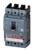
circuit breaker 3VA6 UL frame 150 breaking capacity class M 35kA @ 480V 3-pole, line protection ETU330, LIG, In=100A overload protection Ir=40A...100A short-circuit protection Ii=1.5...12 x In ground-fault protection Ig=0.2...1 x In, tg=0.1/0.3s without connection
