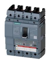
Circuit breaker 3VA6 UL Frame 150 breaking capacity class M 35kA @ 480V 4pole, Line protection ETU320, LI, In=100A overload protection, 100% rated Ir=40A...100A Short-circuit protection Ii=1.5...12 x In N conductor protection adjustable (OFF, 50%, 100%) without connection
