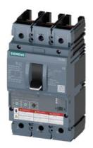
Circuit breaker 3VA6 UL Frame 150 breaking capacity class M 35kA @ 480V 3-pole, Line protection ETU320, LI, In=100A overload protection, 100% rated Ir=40A...100A Short-circuit protection Ii=1.5...12 x In without connection
